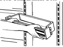
**To remove bins:** Lift bin straight up until mounting hooks disengage.
